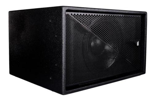
The Hawk Solo 12 is a low frequency loudspeaker featuring a 12" (320mm) transducer with a 3" (76mm) voice coil. It has a flared port to assist laminar air flow and maximize acoustic output. Two Neutrik® NL4 SpeakON $^{\rm M}$  sockets are fitted to a recessed connector dish, allowing the Solo 12 to be placed flush against a wall. The connectors are wired in parallel, which enables up to four speakers to be connected to a single amplifier channel, reducing install cost and complexity.
